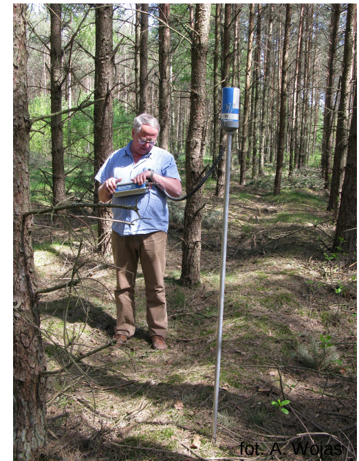
Annual surveys of TMI, proton magnetometer, 0.1nT sensitivity.
